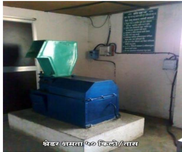
Shredder at Nature in Need Disposal Center Capacity 50 kg. per hour
